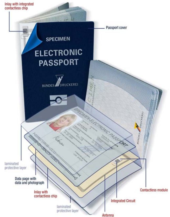
► The contactless chip can be integrated into either the cover page or the data page.
